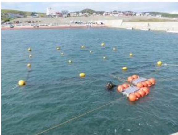
Repellent equipment installed in a floating cage (before improvement)
